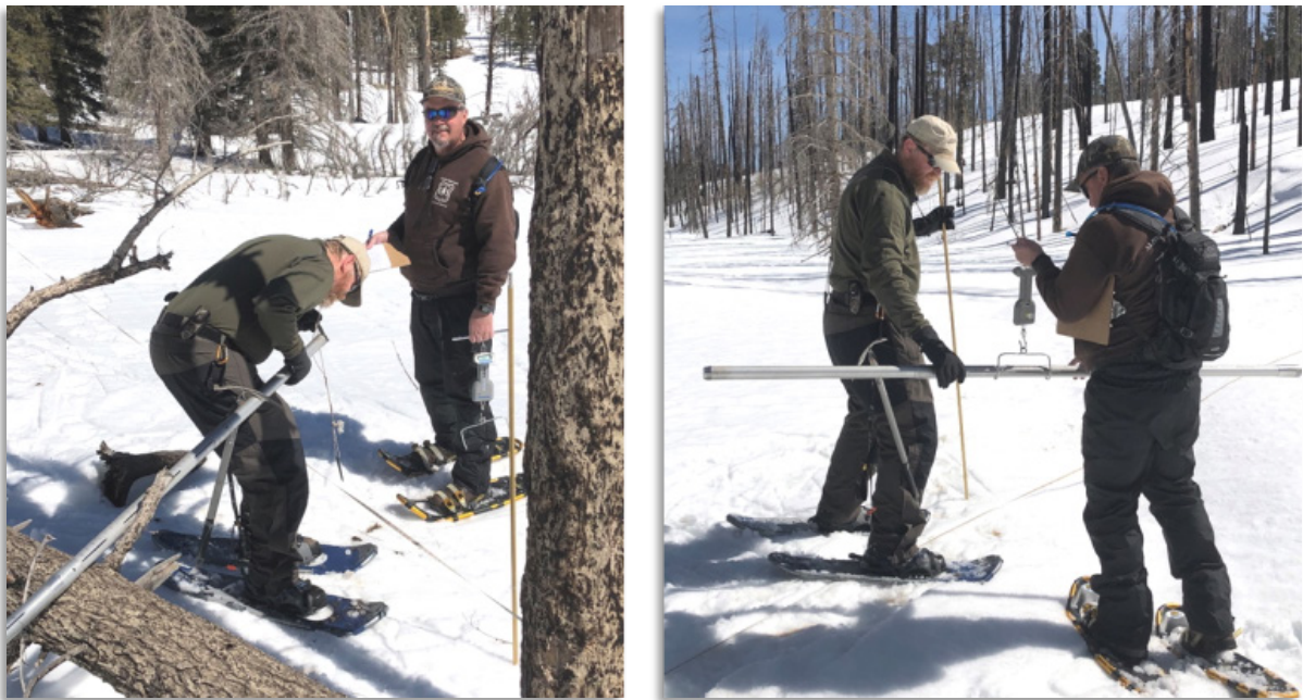
Figure 39. Snow sampling by scientists Chris Johnson, USFS (retired) and Tom Vanzant, NRCS, following the Wallow Fire. Apache-Sitgreaves National Forest, AZ. Photo: Joel Biederman.
