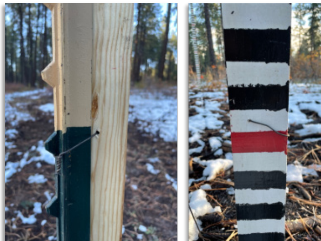
Figure 32. Photos illustrating a baling wire method of attaching snow stakes to T-posts. Photo: Seth Arens.
