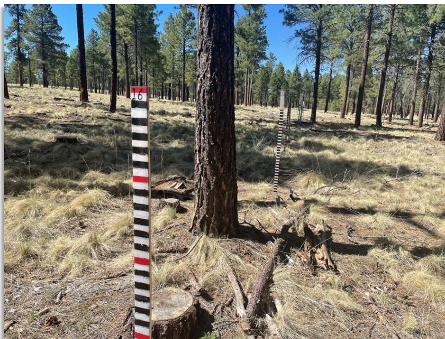
Figure 34. Snowtography transect installed and ready for snow. Photo: Joel Biederman.
