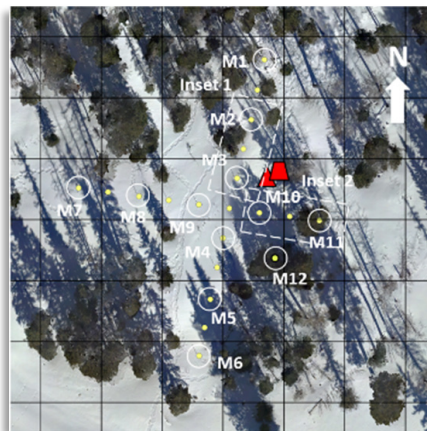
Figure 9. Typical snowtopography station with transects oriented N-S and E-W to capture snow variability under sun, shade, and wind conditions in the forest. The grid cells are 10 meters square. Yellow dots indicate snow stakes 5 meters apart and red shapes indicate a data logger and solar panel. (Some systems have integrated data loggers and solar panels.) Source: Willem van Leeuwen, Arizona Remote Sensing Center.
