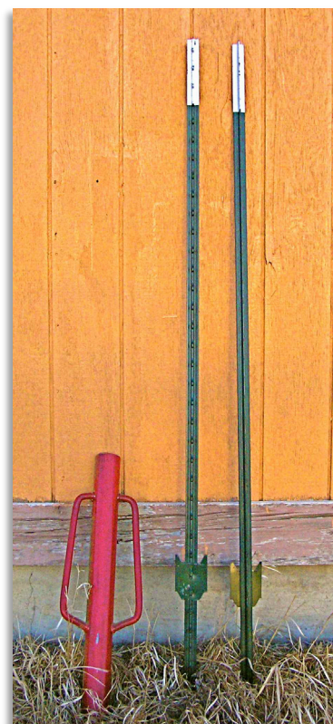
Figure 18. A post-pounder and T-posts. Photo: Montanabw - Own work, CC BY-SA 4.0.
