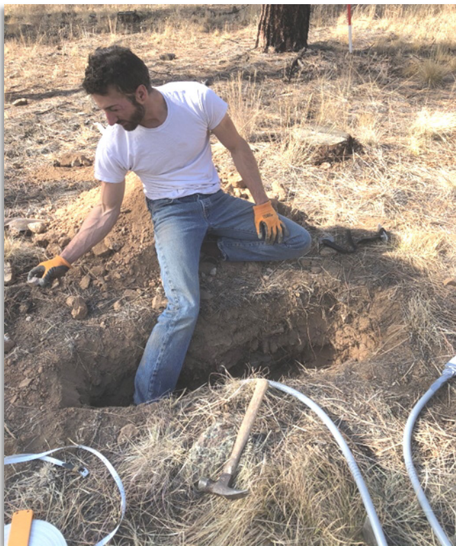
Figure 42. Adam Belmonte, Northern Arizona University, installing soil moisture sensors that have been fed into flexible conduit and sealed with heavy duty duct tape at Ft. Valley, AZ. Photo: Joel Biederman.
