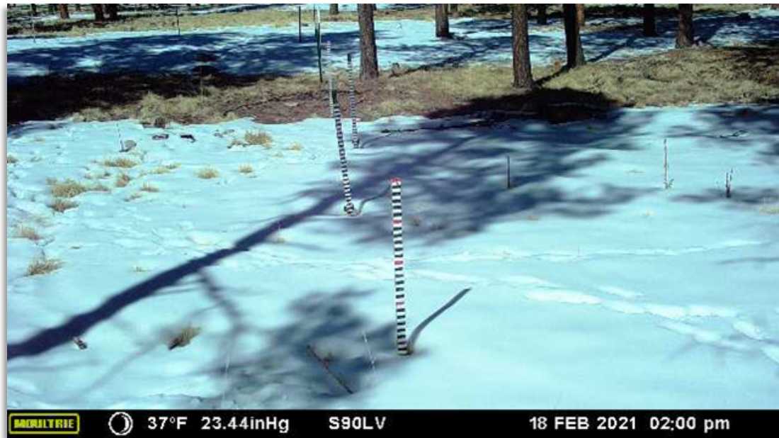
Figure 3. Photo of snowtography stakes taken by a snowtography camera. Source: Arizona Remote Sensing Center.
