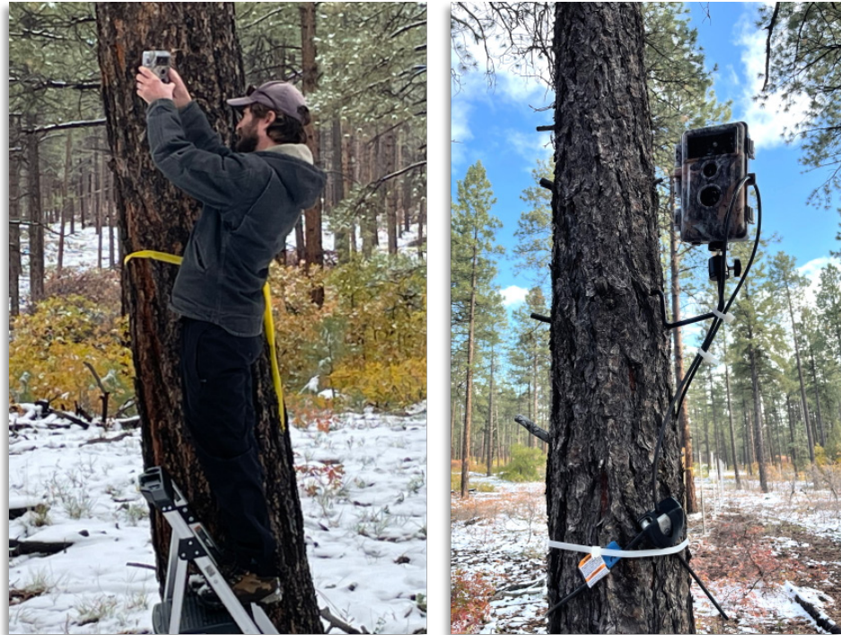
Figure 29. Left: Danny Margoles installing a camera. Photo also shows forestry flagging tape used to mark the tree during planning. Right: Installed camera. Photo also shows the camera mount, cable lock, and zip tie used to secure the cable. San Juan National Forest. Photo: Seth Arens.
