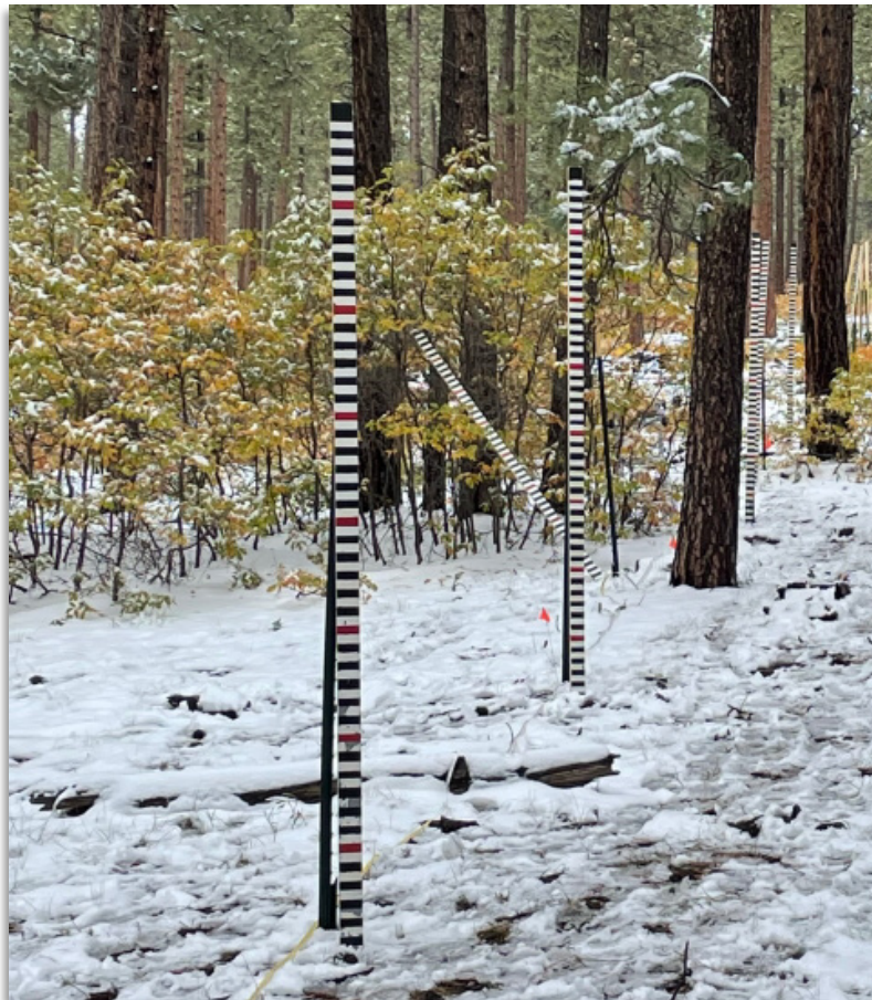
Figure 28. Snow stakes leaning on T-posts to check alignment with a snowtopography camera. Photo also shows transect line (yellow tape) and stake locations (flags). San Juan National Forest. Photo: Seth Arens, Western Water Assessment.
