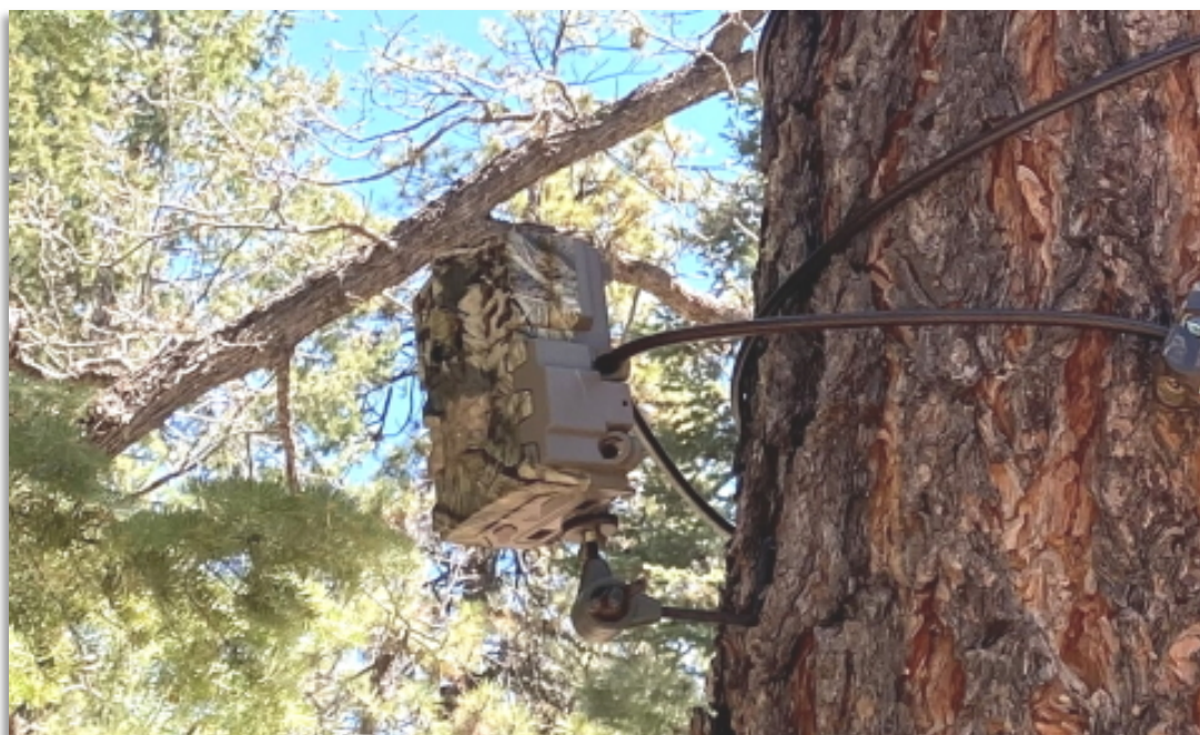
Figure 4. Snowtography camera mounted on a tree. Photo: Patrick Broxton.
