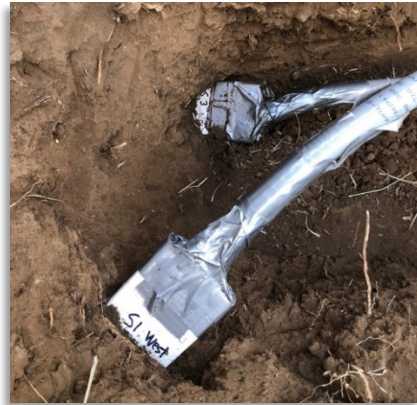
Figure 44. Soil moisture sensors inserted horizontally into a trench face, 15 and 30 cm below the soil surface. Note the horizontal offset between sensors to reduce mutual interference. Sensor cables have been fed through flexible electrical conduit for protection from animals. The tape is wrapped so that no portion of the sensor cable is exposed. Photo: Joel Biederman
