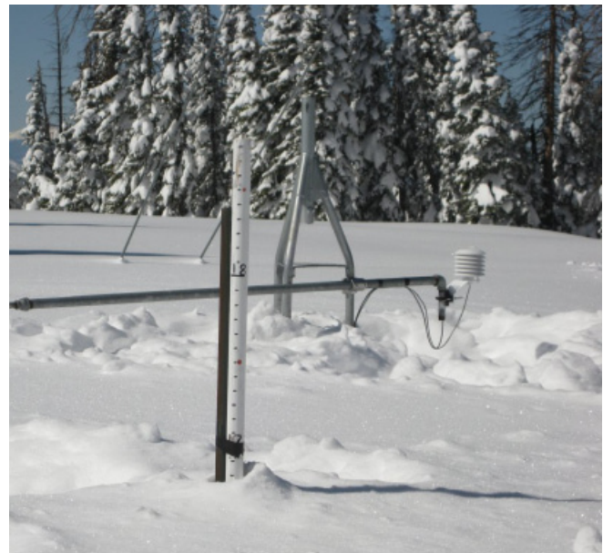
Figure 1. The snow stake and nearly-buried instrumentation at the Tower SNOTEL site near Steamboat Springs, CO, on April 28, 2011. The "17" and "18" on the snow stake mark the height above the ground in feet, indicating a snow depth of 202 inches. (Photo: Mike Gillespie, NRCS Colorado Snow Survey)
