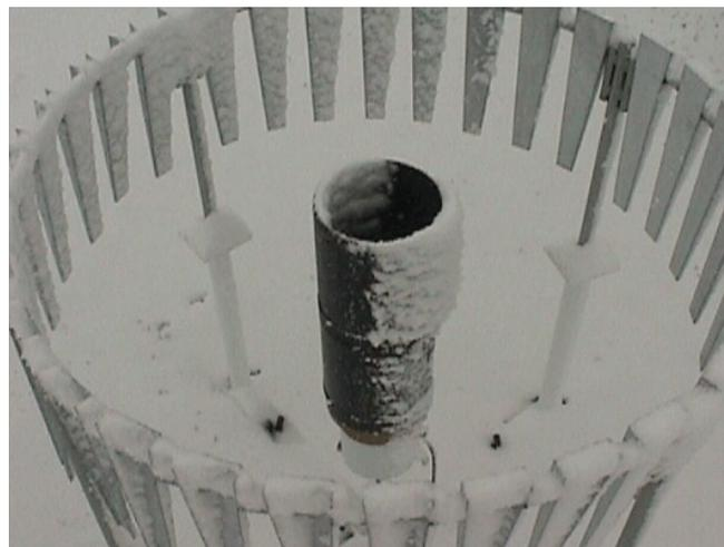
**Figure 1c.** A Tipping Bucket Precipitation Gauge.
