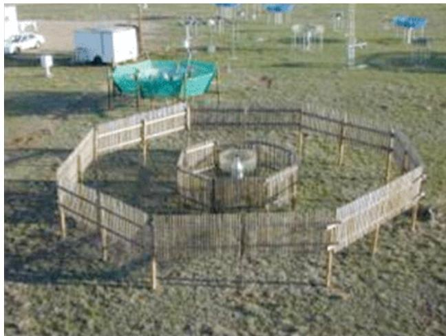
**Figure 1a.** The standard wind shield as set by the WMO at Marshall Field (all photos are courtesy of Marshall Field Winter Weather Group at NCAR).
