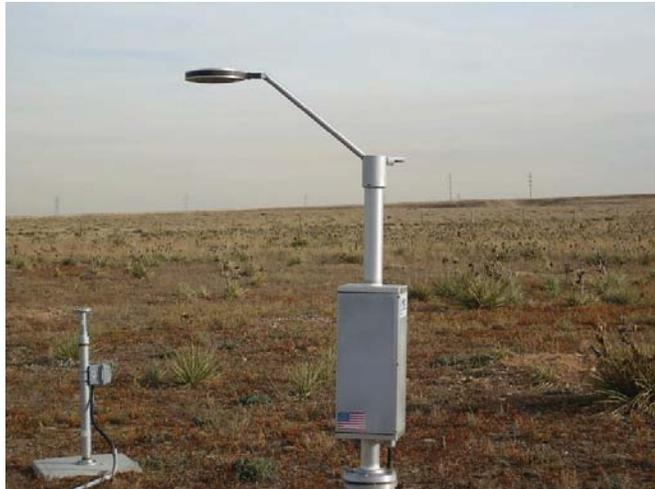
**Figure 1d.** A Hotplate Precipitation Gauge.
