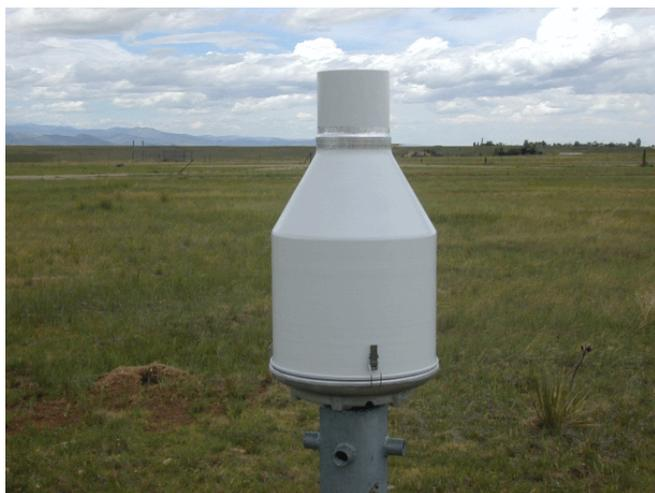
**Figure 1b.** A Geonor Gauge, which is an example of Weighing Precipitation Gauge.
